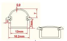
ANODISED 6063 ALUMINIUM RECESSED **EXTRUSION FOR EXCELLENT HEAT** DISSIPATION. COMES WITH MOON/FLAT POLY CARBONATE DIFFUSED **COVER FOR SPREAD** LIGHT EVENLY. GREAT SMART LOOKING. SOLD IN 1m 2m AND 2.4m LENGTHS.
