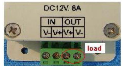
Load output interface: Adopt male and female connector with screw
