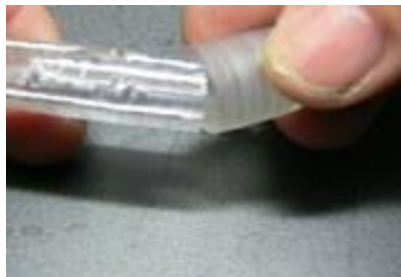
Use silicon in the END CAP to seal from moisture.
