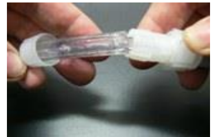
Push connector firmly and deeply into copper wires with pins.
