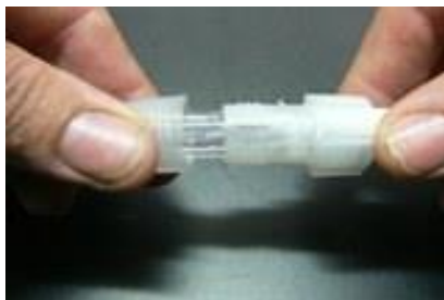
Screw together after connector pins are in place.
